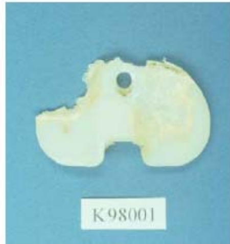
Worn UHMWPE component of total knee replacement.
