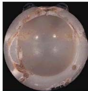
Worn UHMWPE cup of total hip replacement.
