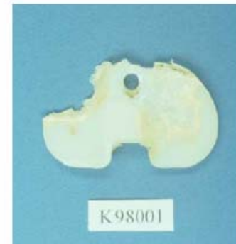
Worn UHMWPE component of total knee replacement.
