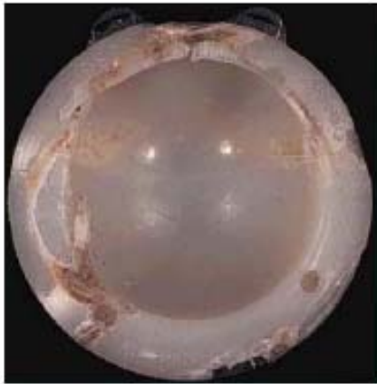
Worn UHMWPE cup of total hip replacement.
